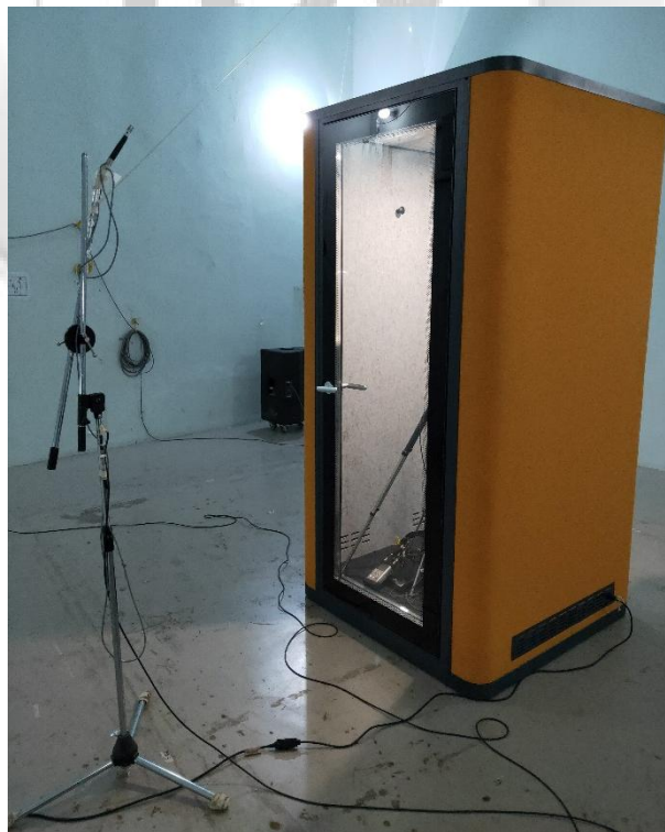
Figure 2 : Test setup of phone booth inside the reverberation room
